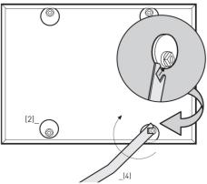
Ready made frame and adjusting screws seen from behind
