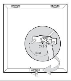
Screw the special fittings (1) onto the wooden frame as shown above using pan-head screws (2).
