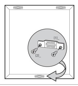
> 02 Fastening the screw locking devices
